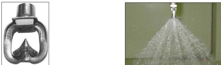
Figure 8 Sprinkler used in PRISME Integral tests (PRISME 1 Project)
