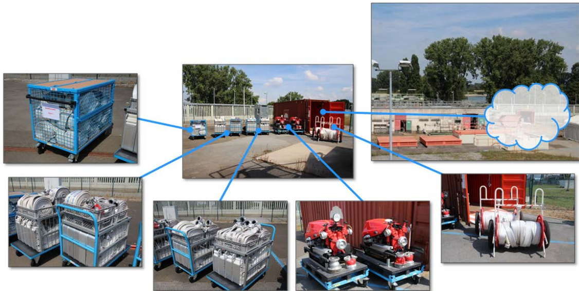
Figure 7 Fire emergency container
