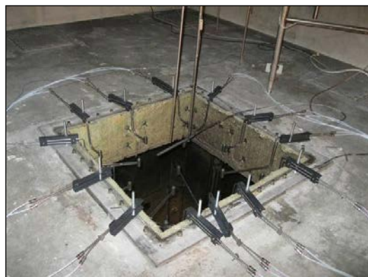
Figure 12 Set of 13 bi-directional McCaffrey-type pilot tubes at horizontal opening
