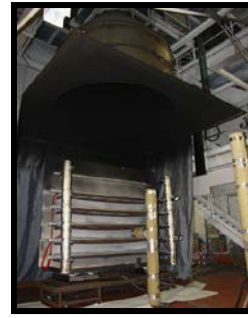
Figure 14 Cable trays device for CFSS fire tests (right: five trays with cables; left: cable trays under calorimeter)
