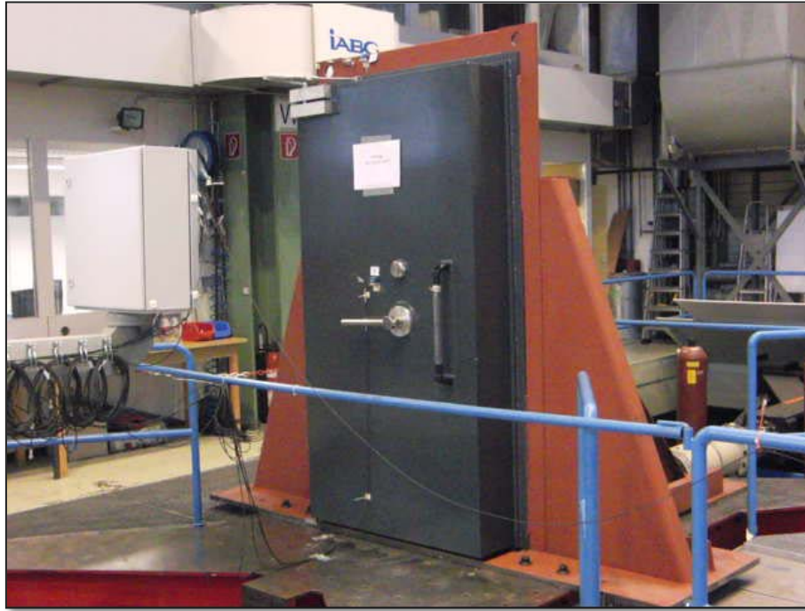
Figure 5 Seismic qualification of a security door
