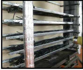
Figure 14 Cable trays device for CFSS fire tests (right: five trays with cables; left: cable trays under calorimeter)
