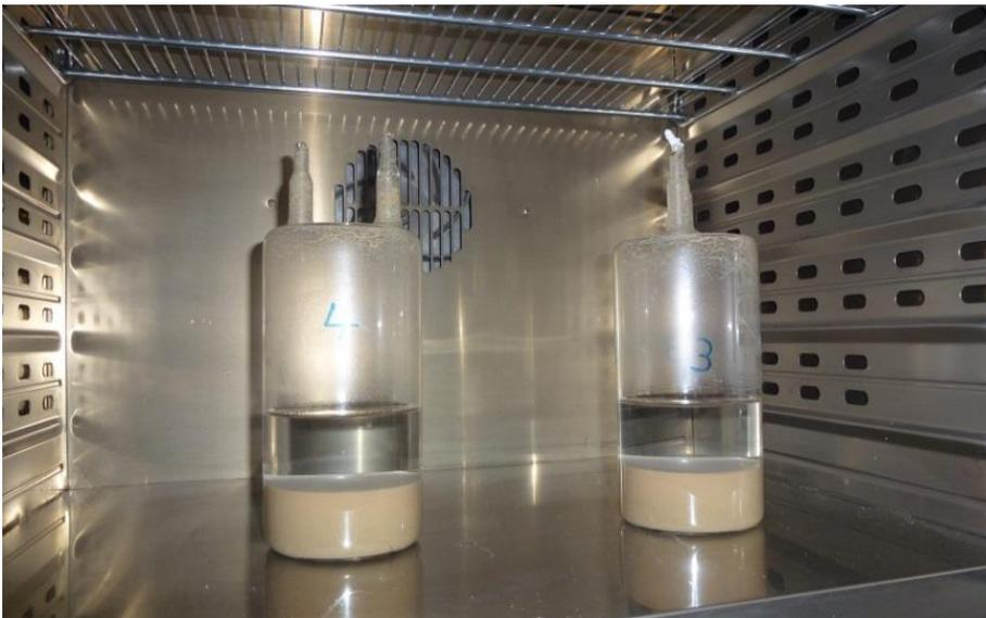
**Fig. 2.2** Bentonite B11 powder after 7 months of reaction with a saturated NaCl- $\text{CaSO}_4$  cap rock solution at a temperature of 90°C.
