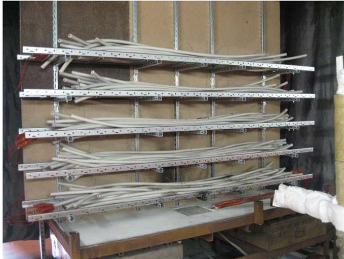
**Figure 2** Picture of the cable trays and loose cable arrangement of the PRISME 2 CORE-1 test before ignition
