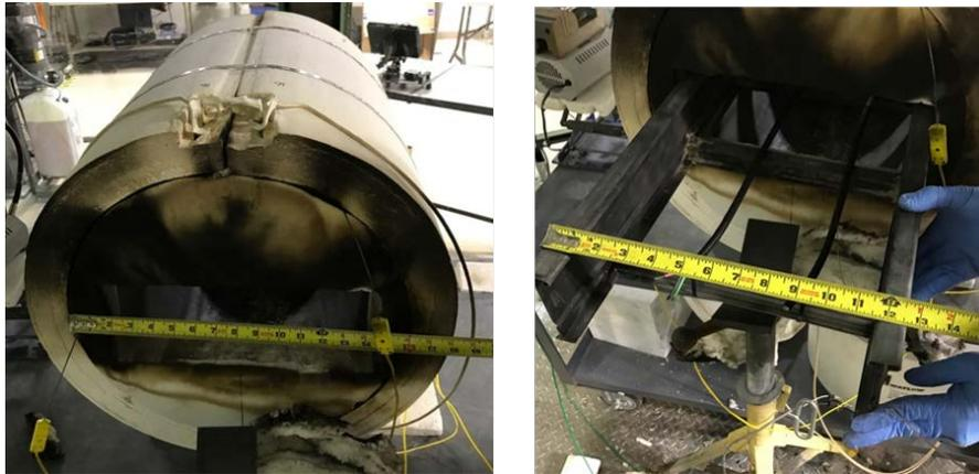
**Figure 9** Picture of cable test setup (left) and ceramic heater (right)
