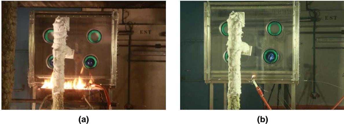
**Figure 1** Ignition phase with (a) a 50 kW wide rectangular burner and (b) a 0.1 kW point burner
