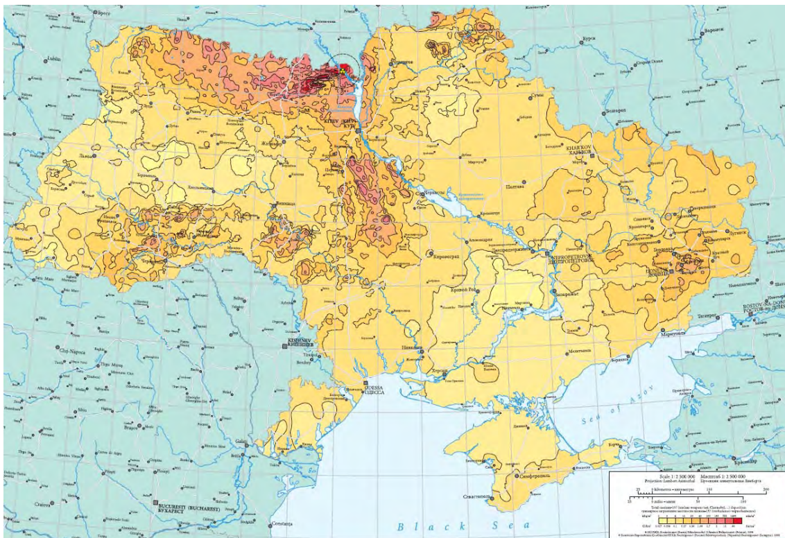
Figure 4-17: Total Cs-137 deposition on the territory of Ukraine (nuclear weapon-test fallout and ChNPP accident) /EEC 98/
